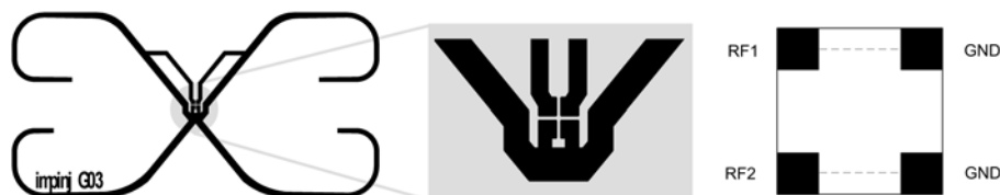
Figure 3-5: Two single-ended connections established for dual dipole antenna. Impinj Jumping Jack™ shown (L) with antenna trace detail (C) and corresponding chip/antenna connections (R).
