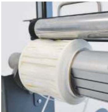
This pressing roller (shown here) positioned above the waste core holder facilitates the matrix removal from the die-cut roll, reducing the risk of tearing and ensuring more precise operation of the machine.
