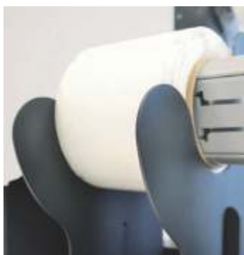
Adjustable guides to obtain the perfect finished rolls.
