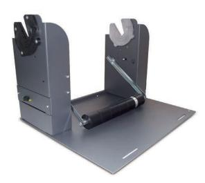
Our range of motorized core holders can handle labels up to 240mm wide and rewind or unwind rolls having outside diameter up to 250mm (contact us for the availability of different outside diameter). Rolls are rewinded/unwinded onto a 3" core holder and the possibility to adjust the sense of rotation, clockwise or counterclockwise, allows to rewind / unwind labels both face in and face out.
